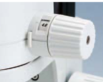
MZ6 zoom magnification changer, and ratchet stops for seven positions
